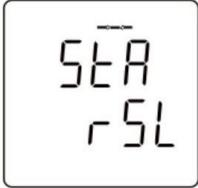
The left figure indicates that no alarm is triggered and the relay is in the connect state.
