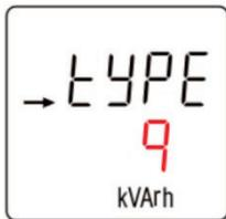
On the left, the pulse output type is import reactive power
