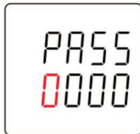
**Passo 2:** Enter the correct user password (**Button 1** to set, **Button 2** for moving). Once you have entered your password, press **Button 2** for 3 second to confirm.
