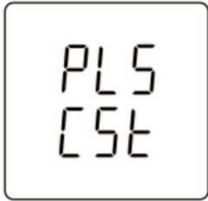
Pulse constant can be set: 1, 10, 100, 1000 imp/kWh(kvarh), default is 1000 imp/kWh(kvarh).
