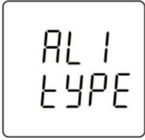
The setting screen of alarm monitoring object of **channel 1**.
