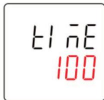
Click **button 1** to select the pulse output width. Press **button 2** for 3 second to confirm the setting. The power meter will save the setting value and exit the setting state. Press **button 1** for 3 second to exit the setting state without saving the setting parameters.
