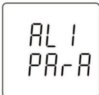
Alarm parameter setting menu for **channel 1**. Press **button 2** for 3 seconds to access the alarm parameter selection screen.
