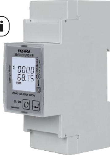
The 1SDSD05CEM2WIFI digital energy meter records energy consumption in single-phase systems. In the presence of a Wi-Fi network, it can be connected to the Internet and consulted via the Perry Smart App installed on a smartphone or tablet. This useful feature allows you to view user consumption even remotely with an easy-to-interpret interface. The relay on the device allows you to disconnect the connected load when a freely settable consumption threshold is reached.
