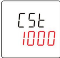
Click **button 1** to select the pulse constant. Press **button 2** for 3 second to confirm the setting. The power meter will save the setting value and exit the setting state.
