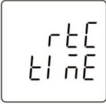
Press button 2 for 3 second to enter the setting state, and the digit of the setting becomes the flashing state. Click button 1 to scroll the page and select the next setting screen. Press button 1 for 3 second to return to the previous level setup menu.
