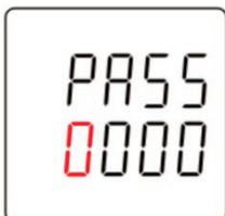
Press **button 1** to set the number. Click **button 2** to move to the right flashing position. After entering the correct password, press **button 2** for 3 seconds to confirm the setting. The instrument will save the setting value and exit the setting state.
