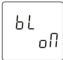
Backlight time can be set: on, off, 5, 10, 30, 60, 120, unit is minute, default is 60 minutes.
