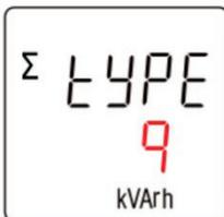
On the left, the pulse output type is total reactive power
