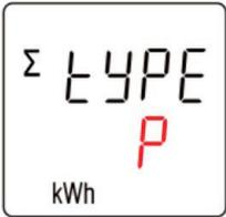
On the left, the pulse output type is total active power
