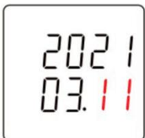
Click button 1 to increase or decrease the number of set bits. Click button 2 can be moved the set bits to the right. Press button 2 for 3 second to confirm the setting. The meter will save the setting value and exit the setting state. Press button 1 for 3 second to exit the setting state without saving the setting parameters.
