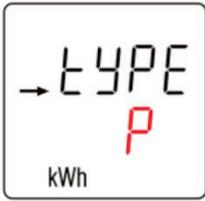
On the left, the pulse output type is import active power
