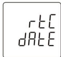
Press button 2 for 3 second to enter the setting state, and the digit of the setting becomes the flashing state. Click button 1 to scroll the page and select the next setting screen. Press button 1 for 3 second to return to the previous level setup menu.
