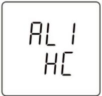
The setting screen of alarm threshold value of **channel 1**.
