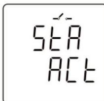
The left figure indicates that the alarm has been triggered and the relay is disconnected.
