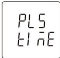
The pulse output width represents the effective duration of the pulse output.
