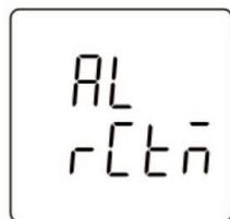
The setting screen of automatic reconnect time for relay.
