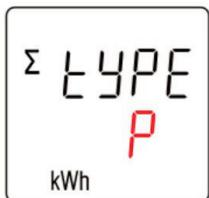
Click **button 1** to select the pulse output type. Press **button 2** for 3 second to confirm the setting. The meter will save the setting value and exit the setting state. Press **button 1** for 3 second to exit the setting state without saving the setting parameters.
